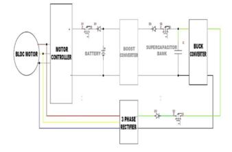
Fig. 6(b). Energy flow in regeneration mode.
