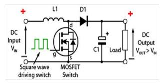
Fig 5: Boost converter circuit diagram
