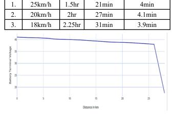
Fig.7: Battery Terminal Voltage Vs Distance before proposed system
