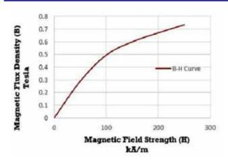
Figure 2. B-H curve of AMT – DAMPRO+ MR Fluid [11]
