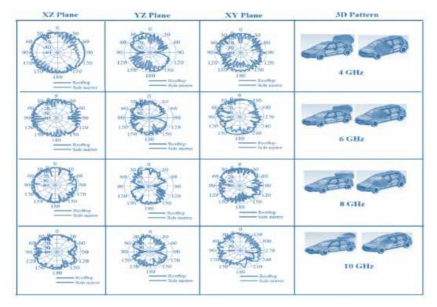
Figure 7: Placement of far-field patterns on a vehicle
