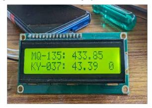
Figure 4: LCD displaying readings of both sensors with voltage as they are operating
