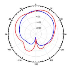
Figure-12 Radiation pattern of SMA
