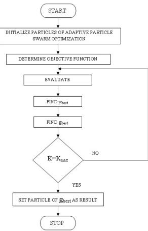
Fig 3. Steps in Adaptive PSO Algorithm
