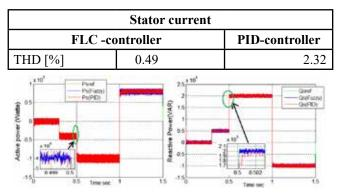
Figure 11. Results of the Power of the chain of wind based on DFIG with Fuzzy controller and PID controller (RT)
