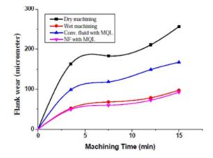
Figure 1B. Tool Flank Wear W.r.t. Machining Time [11]
