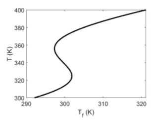
Figure 04: Steady state reactor temperature for parameter set 02
