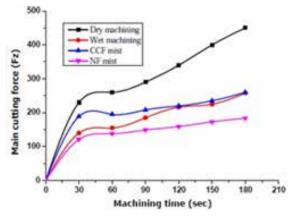
Figure 1a. Cutting Force (Fz) W.r.t. Machining Time [11]
