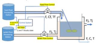
Figure 1: Schematic diagram of CSTR
