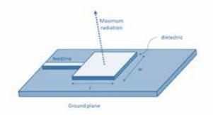
Figure 3: Initial Antenna Element Layout (ROUGH)
