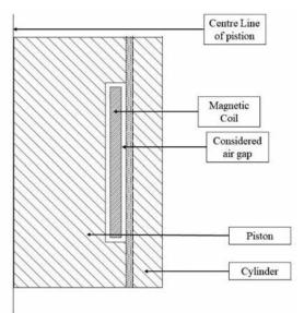
Figure 3.2D Axisymmetric Model Considered for Analysis
