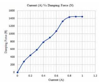
Figure 8. Variation of Damping Force With Respect to Current
