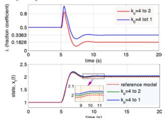
Fig. 4. Adaptive tuned  $\lambda$  optimal and tracking of reference state
