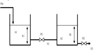
Fig 4. Interacting Two Tank Level Process
