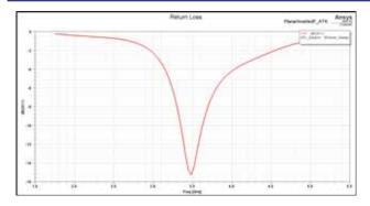
Fig 6. Return loss for EBG based antenna
