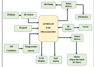
Figure 2. Proposed System Diagram
