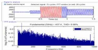
Figure 9. THD of stator current (Fuzzy logic controller)
