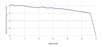
Fig.8: Battery Terminal Voltage Vs Distance after
