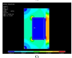
Figure 4. A) 2D Solution of Magnetic Flux Density Obtained for 0.1A Current B) 2D Solution of Magnetic Flux Density Obtained for 0.5 A Current C) 2D Solution of Magnetic Flux Density Obtained for 1A Current
